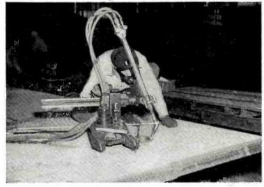
2 WHAT BECOMES OF THE HOLE? In a steel mill, every bit of scrap is collected and re-used. This man is flamecutting armor plate. The steel he cuts out will be re-cycled to the furnace. You can help increase the steel supply if you sell an old tractor, or a plow, or a jalopy, to your nearest scrap dealer.
